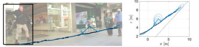
Fig. 7. Scenario V-C2: Results of the proposed filter with the F-RCNN detector, including error covariance ellipses (plotted every 20 ms).
